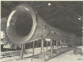
MODEL AIRPLANES MAY BE TESTED AT A SPEED OF 275 MILES PER HOUR IN THIS WIND-TUNNEL
