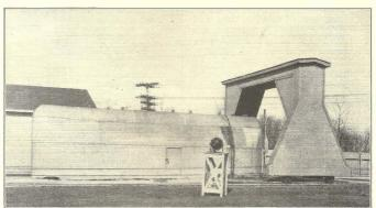
THE PROPELLER-TEST RIG, SHOWING THE "PROP" MOUNTED FOR WHIRLING
